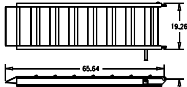
160200 L.H. 160201 R.H. (shown) C-14 only, cleat style, auto-latch, 5 ft. (121703) 4" ch. sides
