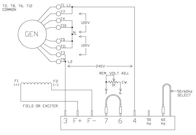
CONNECTIONS FOR 120/240V SINGLE PHASE OUTPUT FROM 3 PHASE GENERATOR
