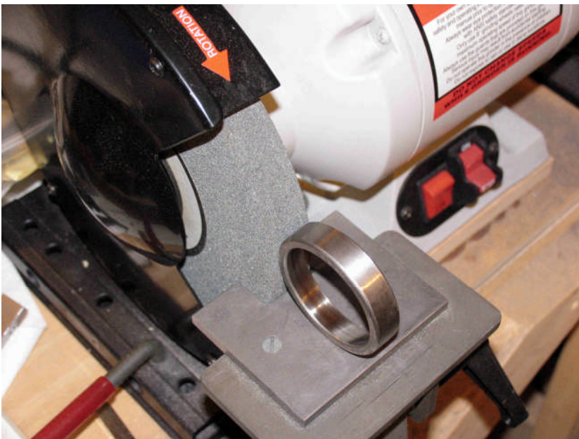
This photo shows how to grind down the old outer race to use as a "Pressor".
