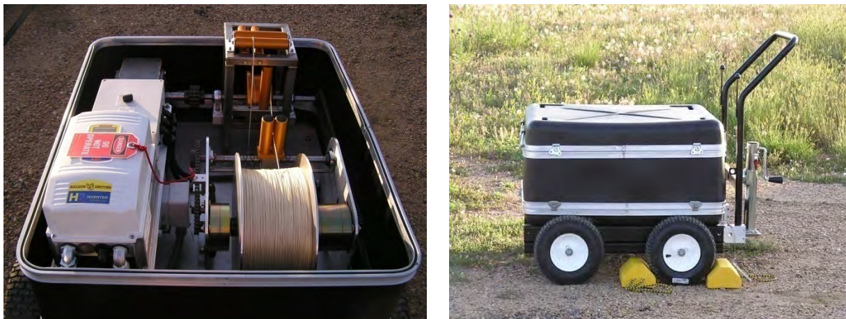
Figure 3: Pictures of the winch with the lid open (Left) and in its transport configuration with push handles, wheels, and jack (Right). The jack is used to remove the wheels and drop the winch on the ground (540lbs/250kg).
