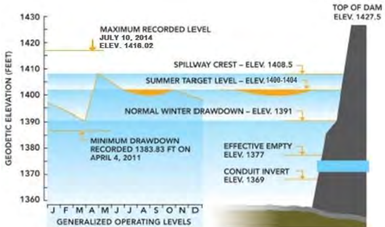
Figure 2: Shellmouth Reservoir operating levels
