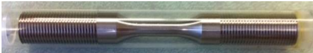
Figure 2.3 Fabricated 316 SS tensile/fatigue specimen
