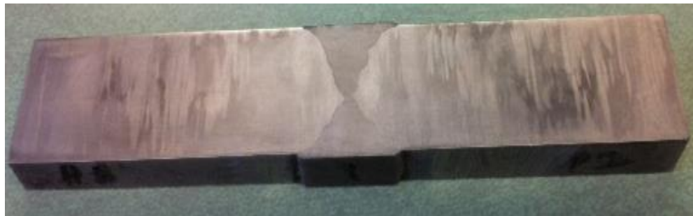
Figure 4.5 Cross section of 316 SS-316 SS welded plate
