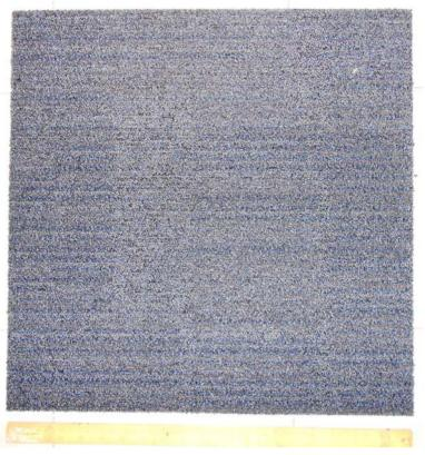
**Figure 2:** The underside of the Interface PET CushionBacRE 780  $g/m^2$  500mm x 500mm Carpet Tiles
