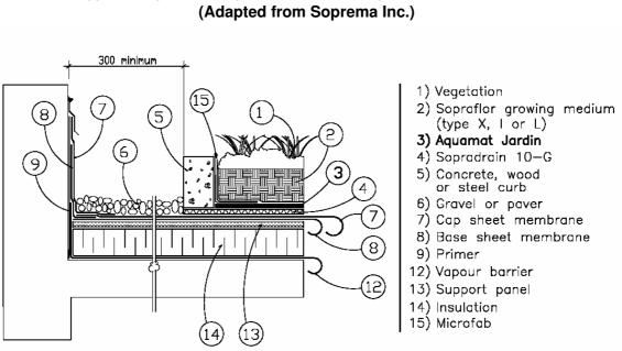
Figure 3.1 A typical Sopranature green roof assembly on conventional roof (Adapted from Soprema Inc.)
