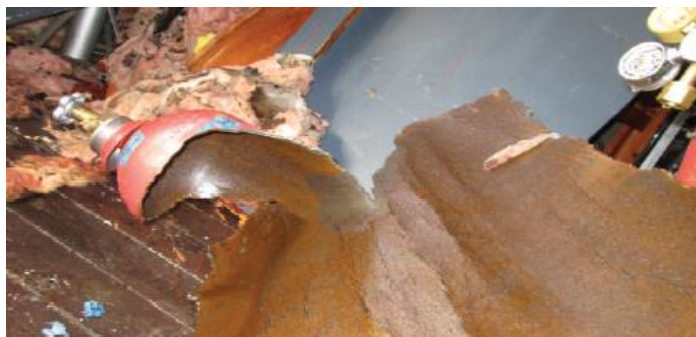
Figure 24: Cylinder embrittlement; note jagged edge and interior surface cracks 55
