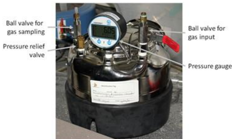
Figure 7: Pressure vessel (1 gallon). The pressure vessel as shown here was equipped with an Ashcroft pressure gauge, a pressure relief valve and two ball valves. When found, the pressure gauge showed an unusually high pressure of 60.5 psig.
