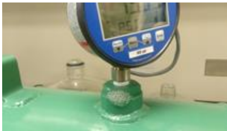
Figure 4: An air leak test done by the postdoctoral researcher using a soap solution indicated air leaks at the gauge and outlet valve reducing bushings (not shown).
