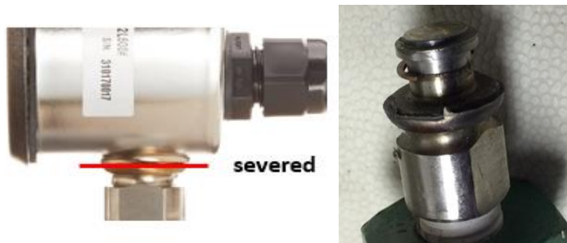
Figures 14 and 15: Pressure gauge stem before (new) and after accident.
