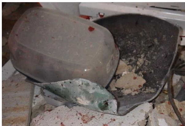
Figure 13: Piece of tank that impacted the autoclave on the floor to left of the biosafety cabinet as found by HFD.
