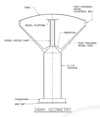
Fig. 1.2a—Common configuration of elevated concrete tanks.
