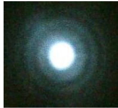
Figure 16.3 - Continuum generated in fused silica
