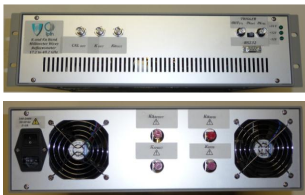
Figure 13.1 - (a) - Front (a) and (b) views of the sub rack containing the TCABr K and Ka reflectometers.
