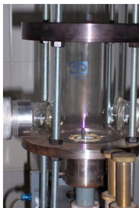
Figure 22.1 - Plasma reactor operated by the axial injection torch
