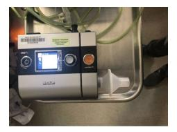
Steps 3 and 4: Connect BOTH inline O<sub>2</sub> feed ports (with 20' oxygen tubing) at VPAP ST outlet
