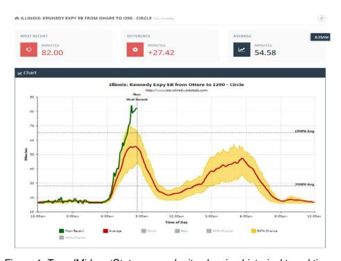
Figure 1. TravelMidwestStats.com web site showing historical travel times
