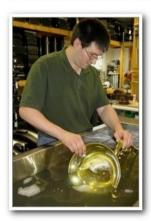
The new, 90-gallon ultrasonic cleaner is large enough to immerse and clean a tuba or several smaller instruments simultaneously. Repair technicians will completely disassemble and prep the instrument before immersion. After an ultrasonic cleaning of the instrument and appropriate parts or components, the repair tech will rinse the instrument before re-assembling and play-testing.
