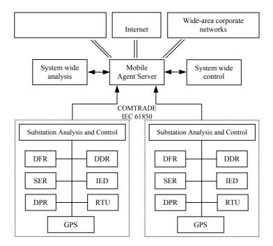
Figure 2: Future trends in the architectures for fault and disturbance analysis implementations.
