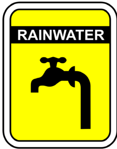
Figure 2: Example of rainwater tank or outlet signage as per AS1319 (AS 1994; AS/NZS 1994)
