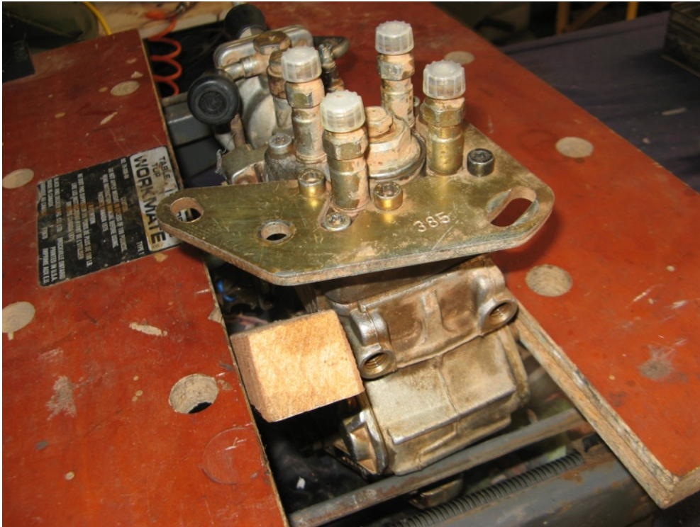
The pump secured vertically in a bench vice
