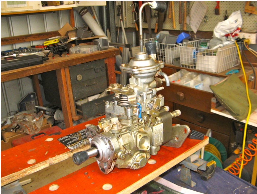
The injector pump complete and ready for refitting
