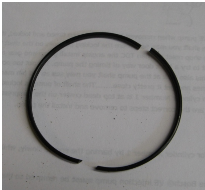
The hardened (and brittle) O-ring which caused the leak
