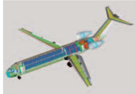
Complete preliminary study of a short to medium haul aircraft with forward-swept NLF wing
