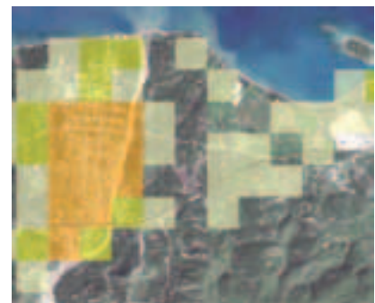
Rapid damage assessment based on emergency maps derived from satellite data; here: Haiti 2010
