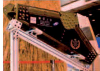
Guide rail for a rear flap (flap track) manufactured in CFRP
