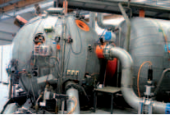
Pressure chamber for human subject research. Rapidly changing pressure profiles can be achieved via high-volume pipes with computer controlled servo valves.
