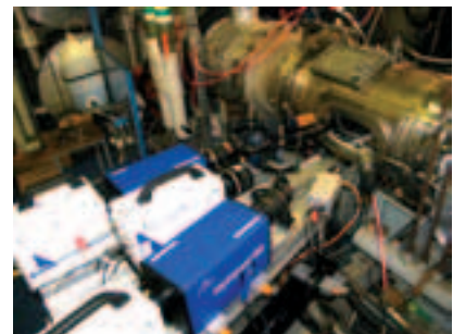
Experimental analysis of ignition process using high-speed cameras in a Rolls Royce test rig
