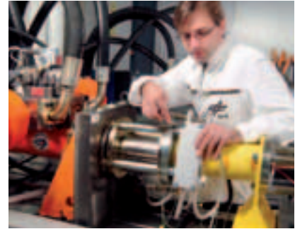
Free-piston linear generator
