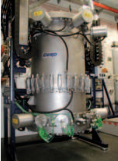
First operation of test rig to characterise SOFC under increased pressure: operation under increased pressure (1-8 bar) Focus: electrochemistry at increased pressure/ operation of SOFC under increased pressure at system-relevant conditions
