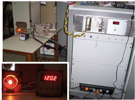
FIGURE 11: The photograph of the developed induction heating power supply. The graphite susceptor heated to 1200°C is shown in the inset.
