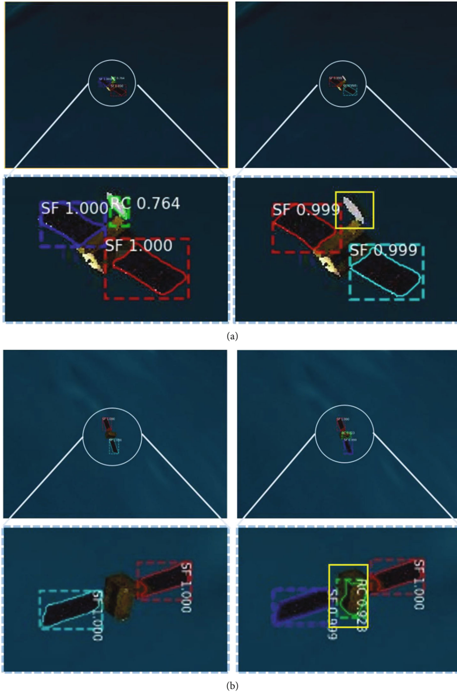
FIGURE 11: Comparisons between the proposed one and Mask R-CNN. (a, b) are the detection results of the two samples, where the left side of each sample is the detection result of RSD, and the right side is the detection result of Mask R-CNN. The bottom row is a close-up of the test results, with the yellow box representing the incorrectly detected part.
