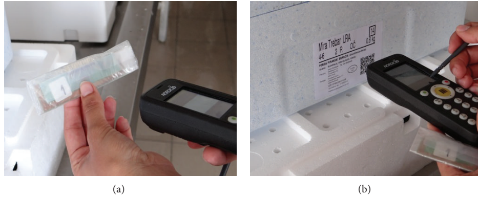
FIGURE 5: RFID-TL (a) is identified; and (b) aggregated with the box.
