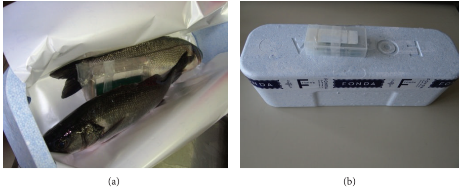
FIGURE 7: RFID-TL (a) is placed between the fish; (b) closed styrofoam box.
