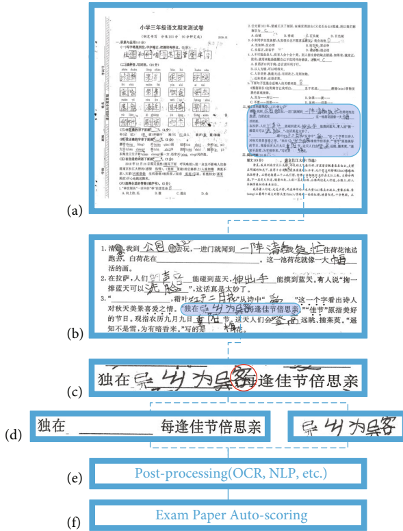
FIGURE 1: Basic process of examination paper autoscoring. (a) A sample examination paper which consists of both handwriting and printed text. (b) A subsection with answers to be scored. (c) Handwriting touches or even overlaps with printed text. The red circle shows an example of overlapping characters. (d) The proposed method targets separation of overlapping Chinese characters into printed text (left rectangle) and handwriting (right rectangle). (e, f) After successful separation is made, postprocessing and autoscoring become feasible.
