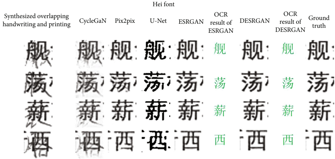
FIGURE 6: Results of separating printed Chinese characters in Hei font. Columns from left to right: synthesized handwritten/printed overlapped data sample in test set and results of separation of printed characters by CycleGAN, Pix2pix, U-Net, ESRGAN, and DESRGAN. The ground truth and OCR recognition results are also provided. U-Net classifies each pixel into one of two categories and generates a binary image.
