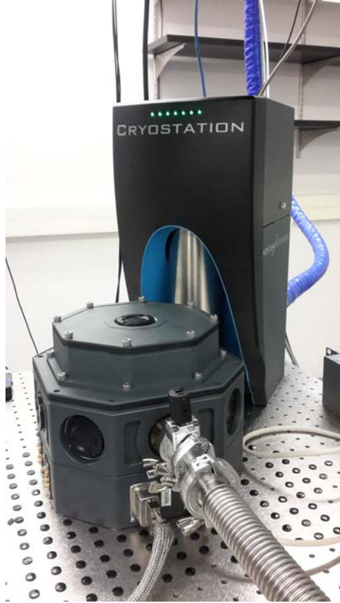
FIG. 4. Image of the sample chamber and Cryostat.
