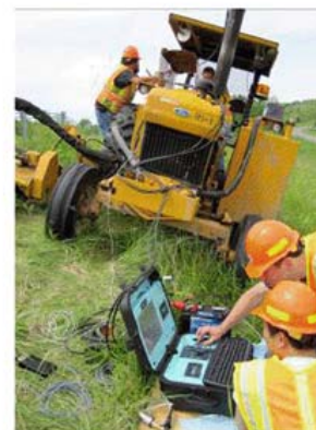
Figure 14. Preparing the setup of emissions equipment on a tractor in real-mowing conditions.
