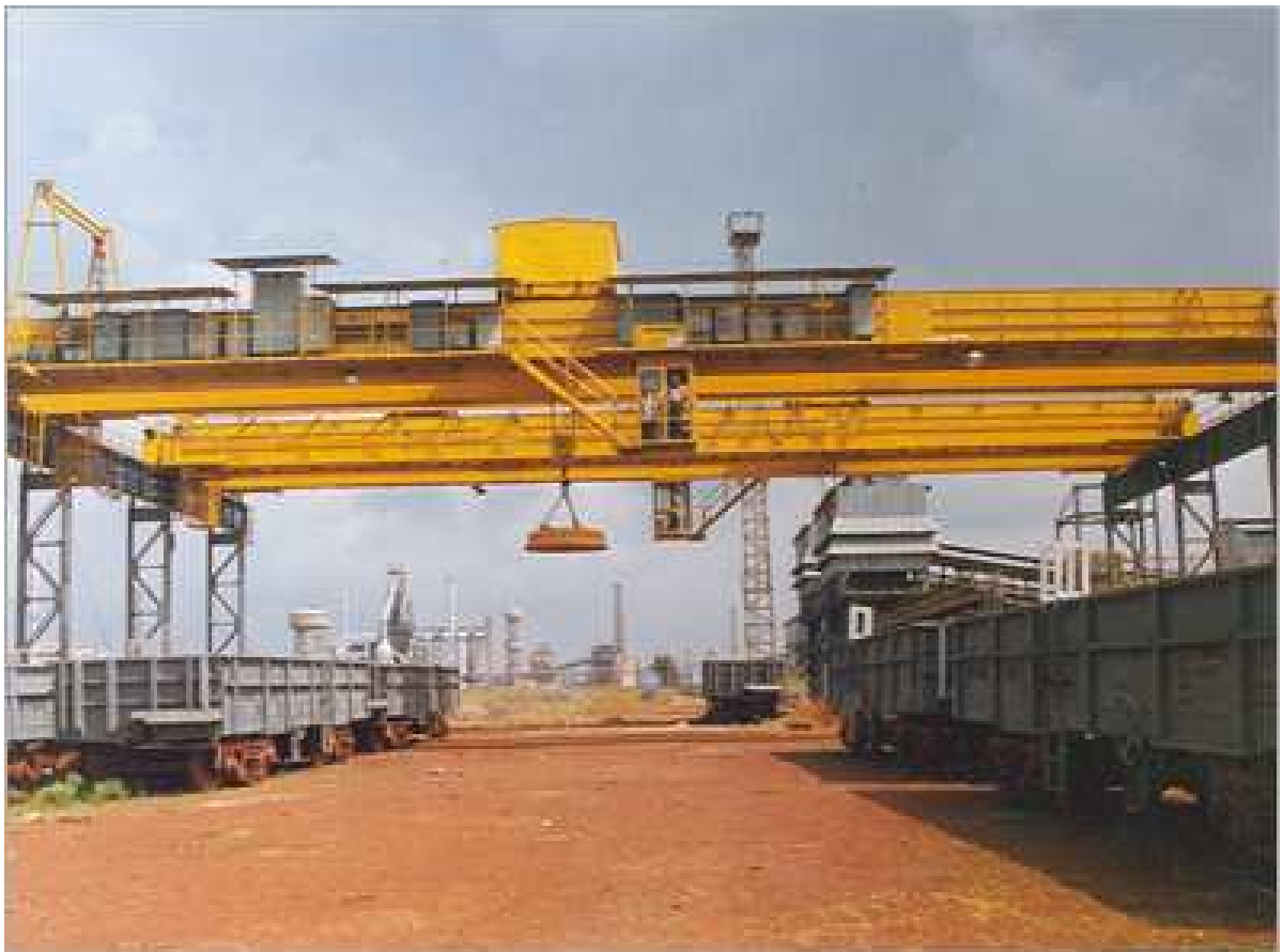
Fig. 1.4 Double girder, magnet EOT crane
