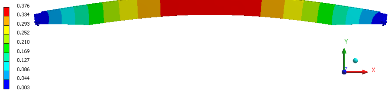
Fig. 6.11 First vertical (Y-axis) modal shape of the crane (first vertical natural frequency f_1=2.44\text{Hz} )
