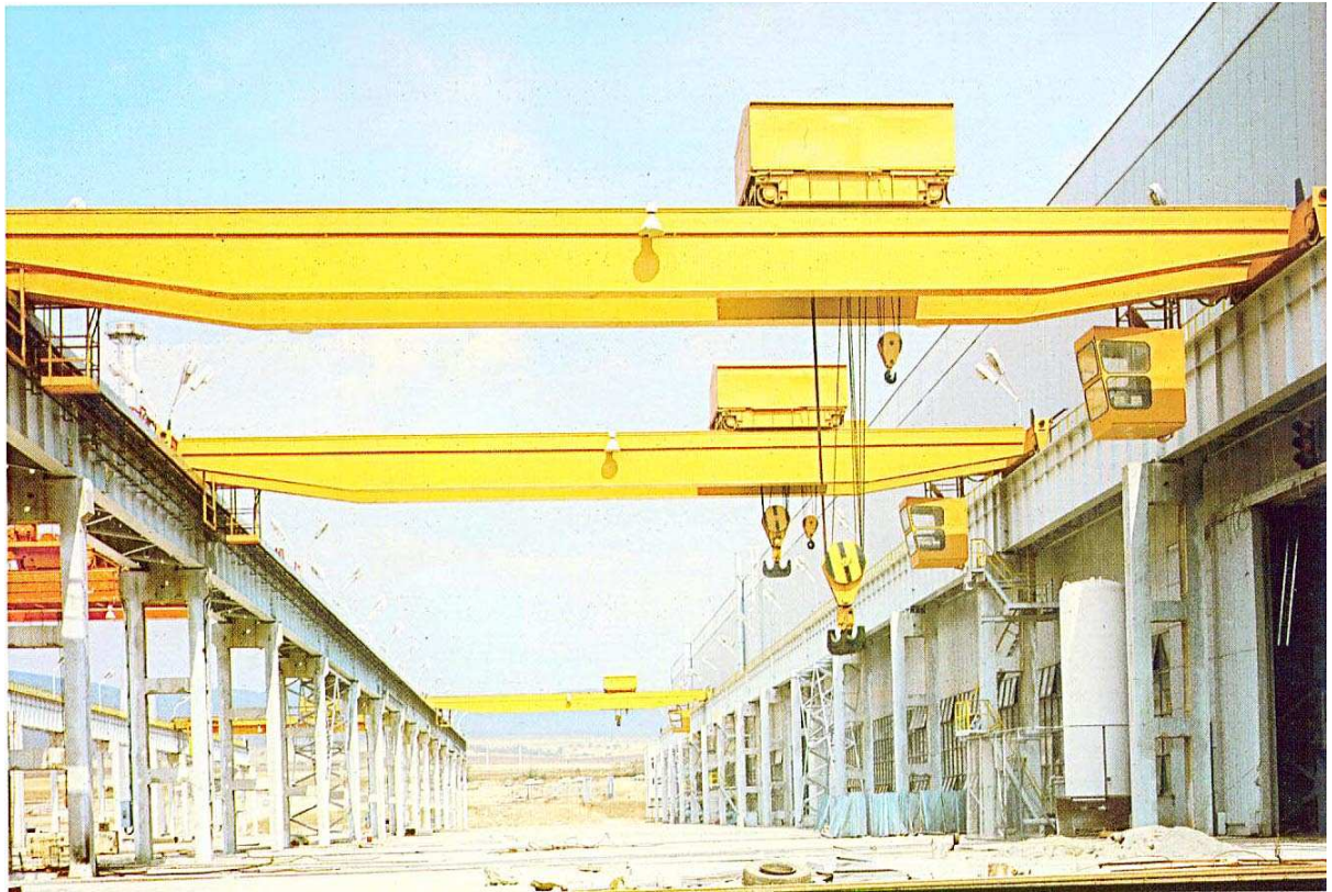
Fig. 1.3 Double girder, general purpose EOT cranes
