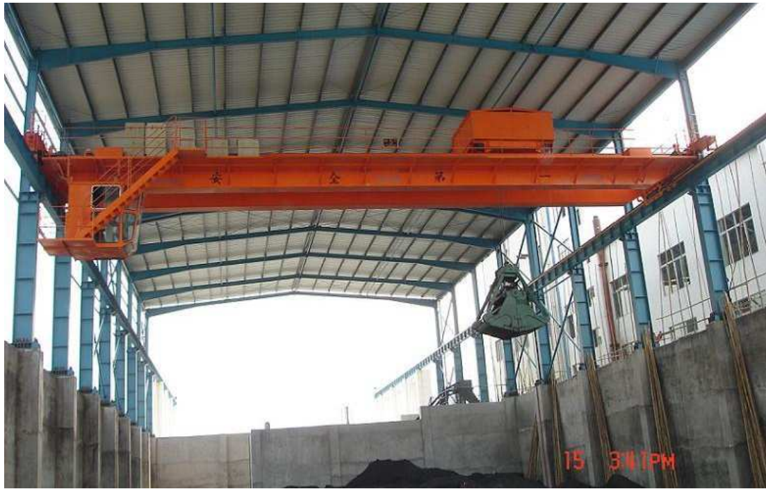
Fig. 1.5 Double girder, grabbing EOT crane
