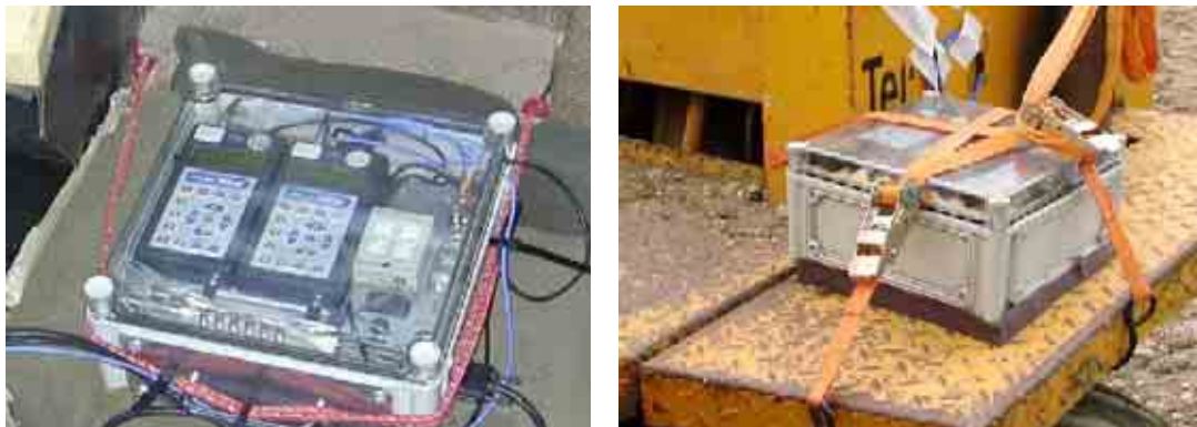
Figure 2.3 Tri-axial 'Floor' accelerometer installation using magnetic mounting
