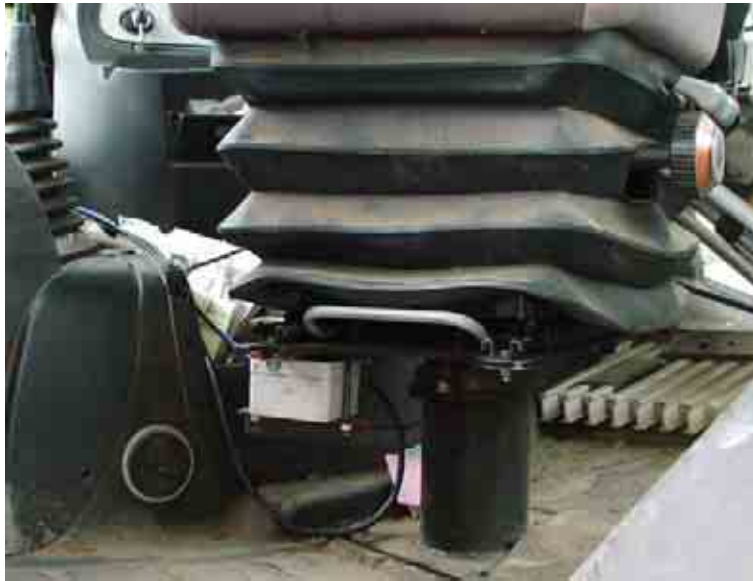
Figure 2.1 'Floor' tri-axial accelerometer configuration (Transducer set 1)
