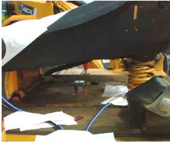
Figure 2.3 Tri-axial 'Floor' accelerometer installation using magnetic mounting
