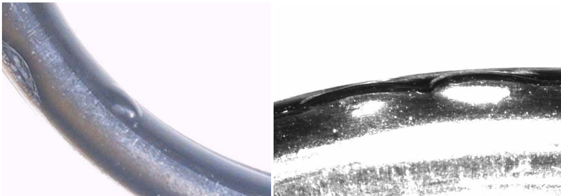
Figure 8 Blisters appear after rapid decompression
