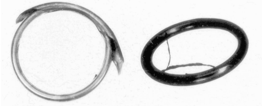
Figure 18 Typical peeling damage to O-ring caused by extrusion
