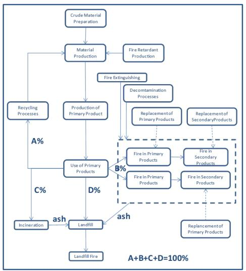
Figure 3: Fire-LCA framework (Simonson McNamee et al., 2011).
