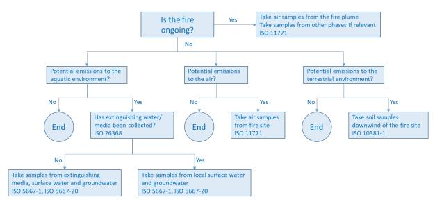
Figure 2: Flow chart designating potential sources of sampling information for emissions from fires. ©ISO. This material is reproduced from ISO 26367-2: 2017, with permission of the American National Standards Institute (ANSI) on behalf of the International Organization for Standardization. All rights reserved.
