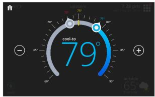
On the Home Screen, touching the cool setpoint indicators on the round temperature band, or touching the **cool-to** button displays the cool menu screen.
