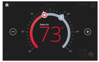
On the Home Screen, touching the heat setpoint indicators on the round temperature band, or touching the **heat-to** button displays the heat menu screen.
