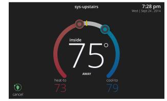
Set heating or cooling setpoints during unoccupied periods.
