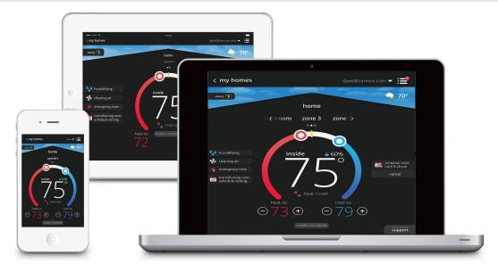
Wi-Fi remote temperature monitoring and adjustment through a home wireless network via desktop PCs, laptops, and apps for smartphones or tablets. Controls on the devices have the same appearance and functions as the touchscreen display, making it easy to make any settings and adjustments.
