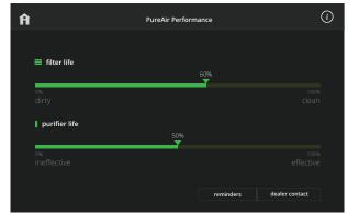
Displays filter life and purifier (UVA lamp/PCO cartridge insert) life status.
