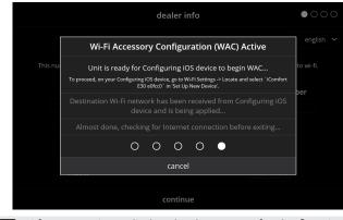
After power is applied to the thermostat for the first time, it displays the iComfort<sup>®</sup> "splash screen" (see page 24), then the Wi-Fi Accessory Configuration (WAC) Active screen for configuring the IOS device will appear on top of the dealer info setup screen.
