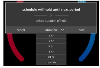
The schedule hold screen is displayed after changing the temperatures on the heating or cooling screens while a schedule is running. Preset 1, 2, 8, 24 hours or custom setting (using the Time Tool) sets and hold the temperature for a preset or custom time period until the next time period setting. Cancel schedule hold button on Home Screen cancels the held setting.
