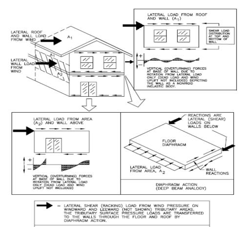
NOTE: WHILE LATERAL LOADS ARE SIMILARLY TRANSFERRED TO WALLS BY DIAPHRAOM ACTION, SEISMIC FORCES ORIGINATE FROM THE TRIBUTARY MASS OF THE BUILDING (I.E., PLAN AREA), NOT THE EXTERIOR SURFACE AREA AS IS SHOWN FOR WIND.
