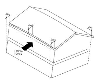
NOTE: IF STIFFNESS OR LOAD IS NONSYMMETRICAL, BUILDING ROTATION OCCURS  $(\bigtriangleup_1 \neq \bigtriangleup_3)$  and Loads are distributed by torsion  $(\bigtriangleup_4 \neq 0)$  as well as by direct shear in the direction of the lateral force. This condition varies but is a reality for most designs.  $\bigtriangleup_2$  is the bending deformation of the horizontal diaphragm (i.e., Roof).
