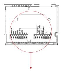
To remove the thermostat backplate: Gently separate the display from the base by pulling first from one side, then the other until the two pieces unsnap. A small screwdriver may be used, very carefully, to start seperating the two pieces.
