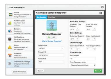
The right column of the ADR configuration page is where the occupant adjusts the operational parameters for ADR. The utility may send up to 3 types of ADR signals to Skyport. These are: 1) Pricing for the cost of energy, 2) An Offset to the occupants' comfort setpoints, and 3) a signal to enforce discrete or Static setpoints.
