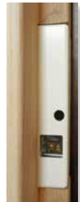
Electronic Interlock (EMDL)
