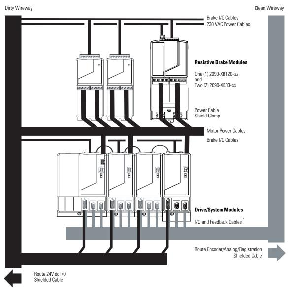
1 If system I/O cables contain dirty (relay, etc.) wires, route these signals with a separate cable in the dirty wireway.
