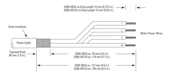
5. Prepare your 230VAC auxiliary power cables (2090-XB120-xx only) by stripping the appropriate length of insulation from the end of the wire. Use caution not to nick, cut, or otherwise damage strands as you remove the insulation.
