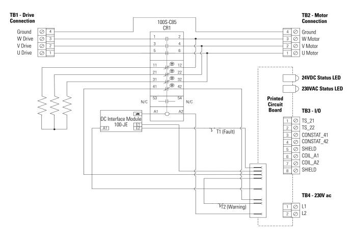
Figure 9 2090-XB120-*xx* Resistive Brake Module Block Diagram
