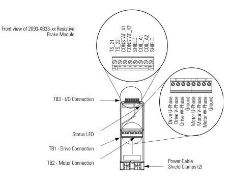
Figure 7 2090-XB120-*xx* Resistive Brake Module Connectors and LED Indicators
