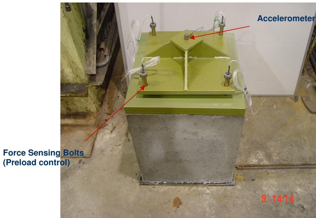
**Figure 3** Innovative rail pad tester
