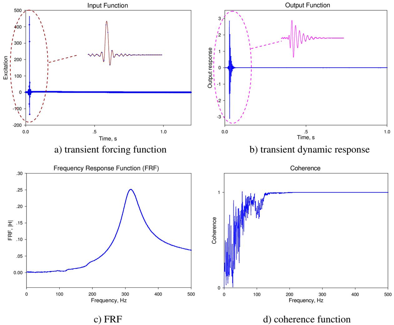
**Figure 5** Vibration response measurements using impact instrumented hammer
