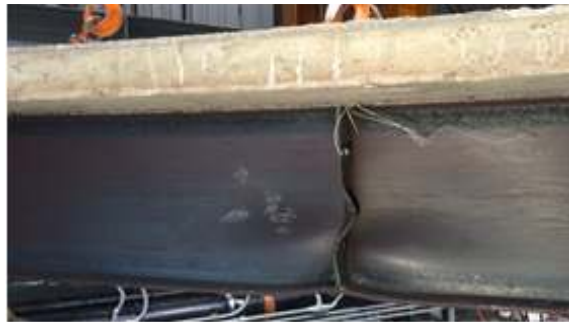
(b) Failure mode of CB2
