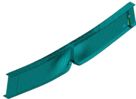
e) Buckling of steel beam (from (d))
