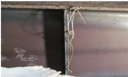
(a) Failure mode of CB1 (Aziz et al., 2015)
