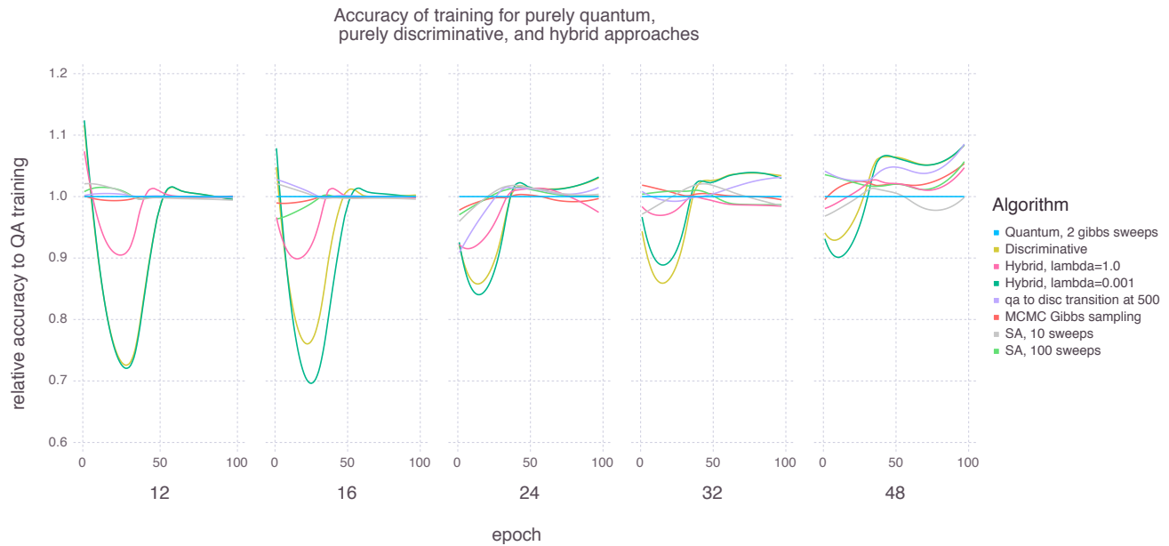
FIG. 10. Comparison of the ratio of various algorithms accuracy against the accuracy of QA training (with 2 Gibbs sweeps) per epoch. Values larger than one imply higher accuracy for the algorithm than QA, below one worse accuracy. This only displays RBM-structured models. Logistic regression and gradient boosted trees dominate RBM-structured models and are not included so as to maximize resolution in the comparison among RBM-structured models. Note: epoch for the tree-based model corresponds to the number of decision trees.
