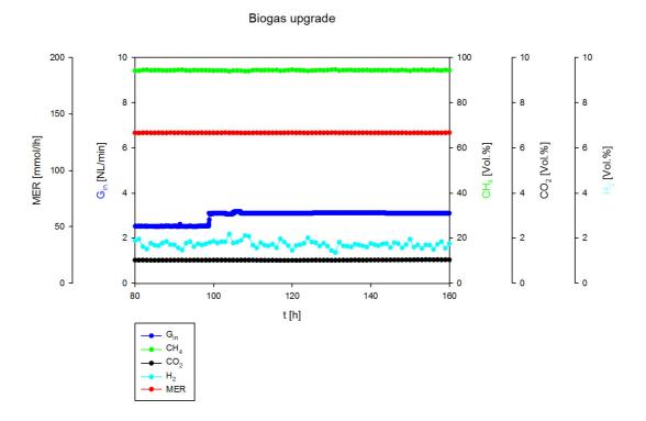
It can clearly be seen that no impact are notifiable compare to a switch to raw biogas as sole  $CO_2$  source of the process. The increase in gassing rate fed to the reactor can be explained by the different volumetric proportion of  $CO_2$  found in the biogas compared to pure  $CO_2$ . The methodology involved into those feasibility studies for evaluating the impact of emission gasses on biological methanogenesis can be found in the literature [24].
