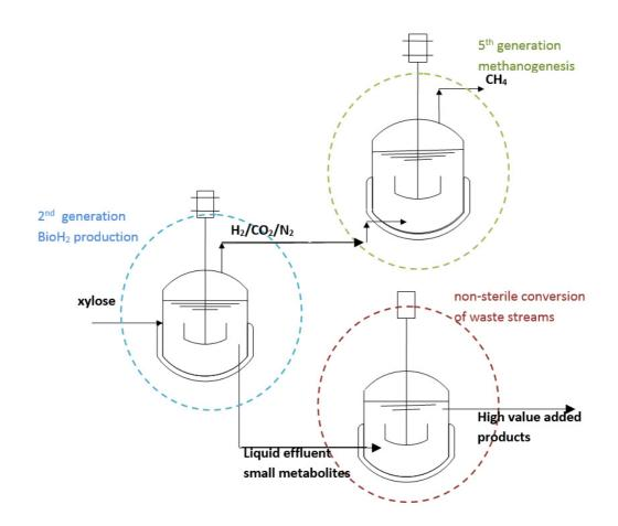
Process integration with extremophilic microorganisms by coupling process streams.
