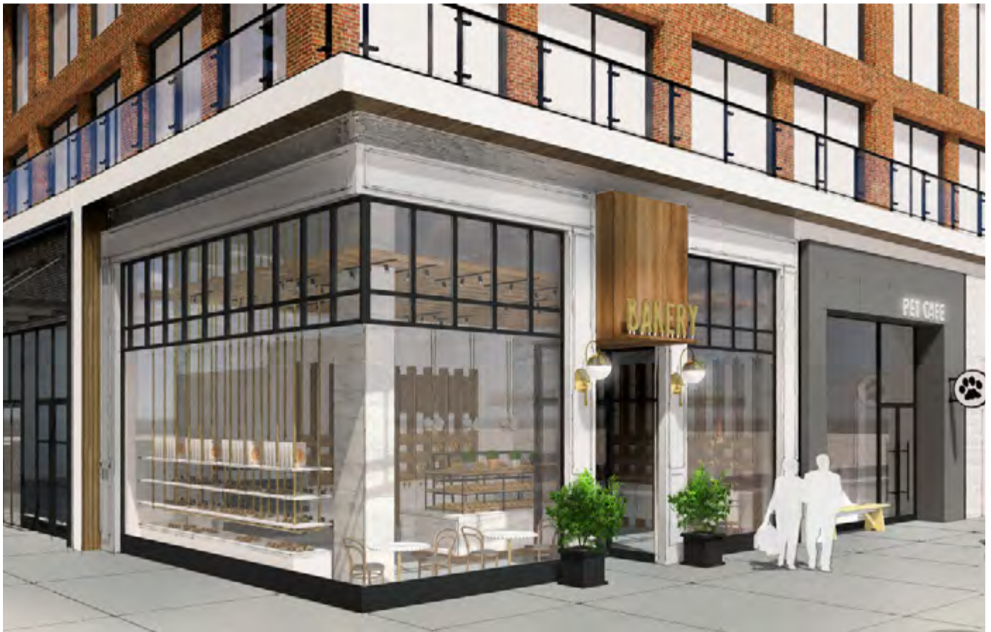
Columns are set back from the retail facade, allowing greater tenant expression.
