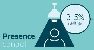
There's no need for lighting to stay set at the same, constant level — especially in staff-only areas or when the store is being cleaned or restocked. With presence detection sensors, it's possible to dim or even turn off luminaires when there's no one around and they're not required. A sensible solution for any environmentally conscious retailer.
