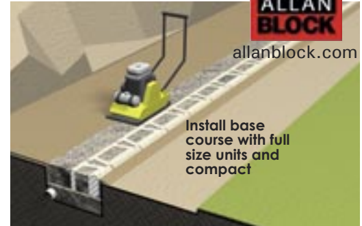
Install base course and compact.
