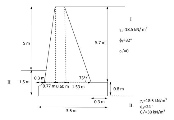
Soil properties: **I**)  $\gamma_1 = 18.5 \text{ kN/m}^3$ ,  $\phi_1 = 32^0$ ,  $c_1 = 0$
