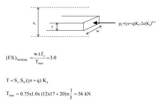
(F.S.)<sub>breaking</sub> =  $\frac{0.075 \text{ x t } \text{ x}3\text{ x}10^5}{56} = 3.0$   $\Rightarrow$  t = 7.46 mm Corrosion rate  $\Rightarrow$  0.025mm/yr. x 50 =1.25mm
