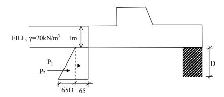
$$\begin{split} &K_p = tan^2 (45 + 32/2) = 3.25 \\ &z = 0 \Rightarrow p_p = 1x20x3.25 = 65 \text{ kPa} \\ &z = D \Rightarrow p_p = (1x20 + 20xD)x3.25 = 65 + 65D \text{ kPa} \\ &P_p = P_1 + P_2 = 65D + 1/2x65D^2 \end{split}$$
