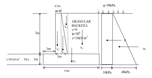
$K_a$ =tan<sup>2</sup>(45-φ/2) For granular backfill⇒ $K_a$ =tan<sup>2</sup>(45-30/2)=0.333 Active pressure,  $p_a$ =(q+γz) $K_a$ -2c√Ka
