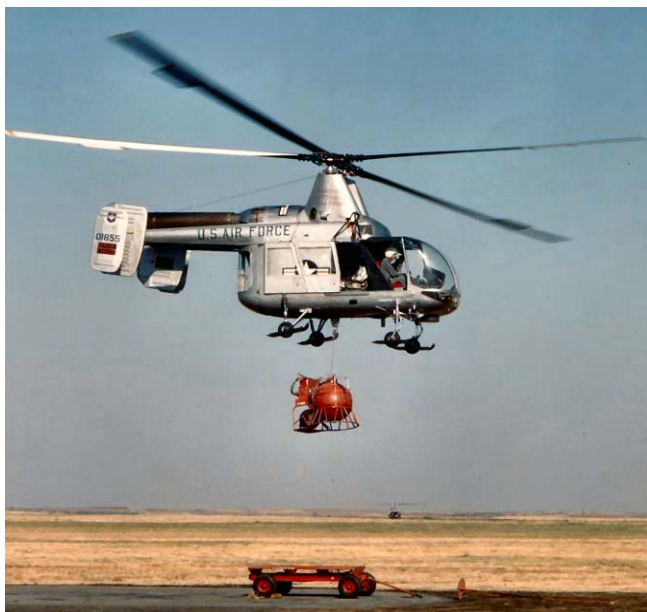
B" Model with Fire Suppression Kit. Rotor-Wash to Aid Rescue Path
