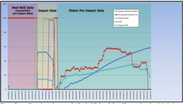
*Figure 7* Data from the example "Locked-Reboot" data file sorted so that it is in its proper memory buffer address order.
