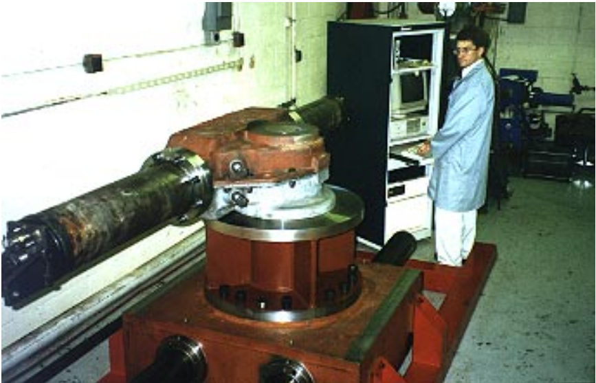
Rotork has extensive testing and quality performance capabilities. The photo above shows an apparatus that tests the torque, life, and performance of spring return and double-acting fluid power actuators.
