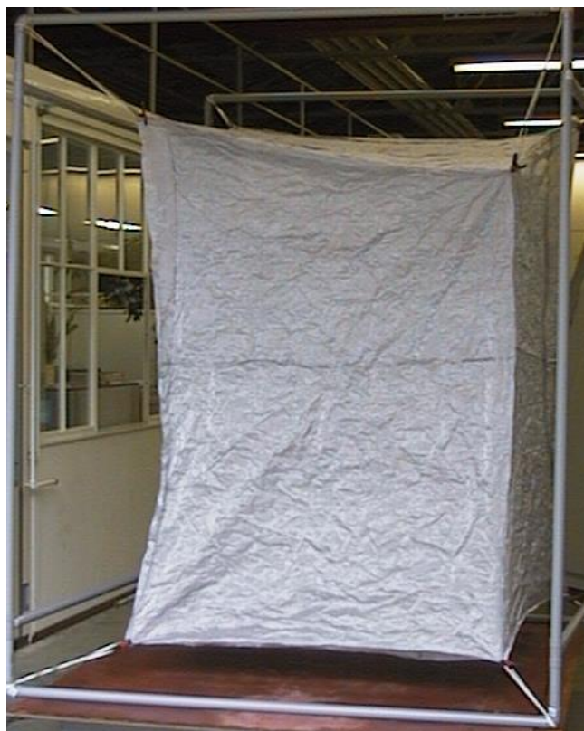
Fig. 12. The Vibrating Intrinsic Reverberation Chamber hanging on strings
