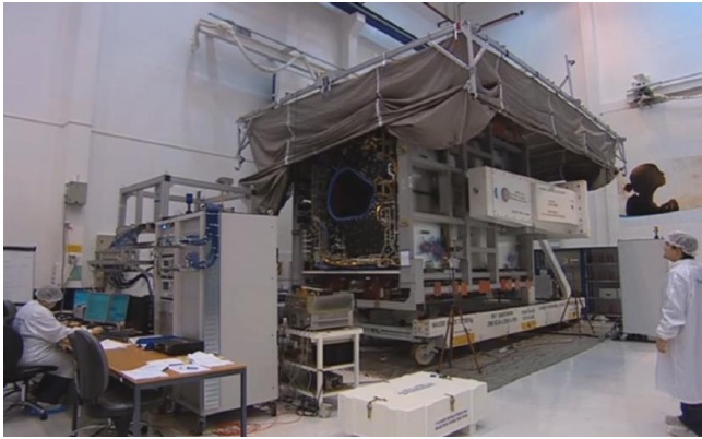
Fig. 13. Using the VIRC for the “sniff and spray test” for satellites. The “sniff and spray tests” are leakage tests on the several thousands of waveguide junctions in a high-tech communication satellite. This test takes normally four weeks with conventional test setups, reduced to few days when the VIRC is used.
