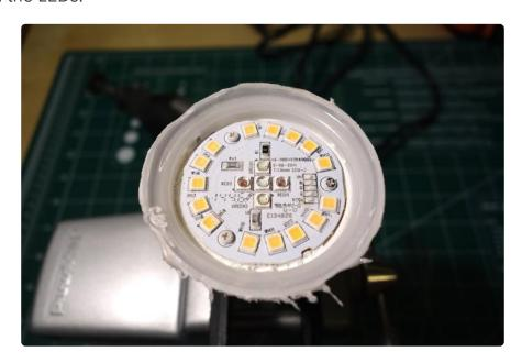
It's interesting to see a ring of white LEDs (soft white actually, somewhere around 3500K I would guess) around the perimeter of the board. In the middle are the colored LEDs, with two green, two red, and one blue LED. Presumably when the bulb shows pure white it turns on the outer white LEDs to have a more pleasing color as the red, green, and blue LEDs would be colder and less pleasant for indoor lighting.
