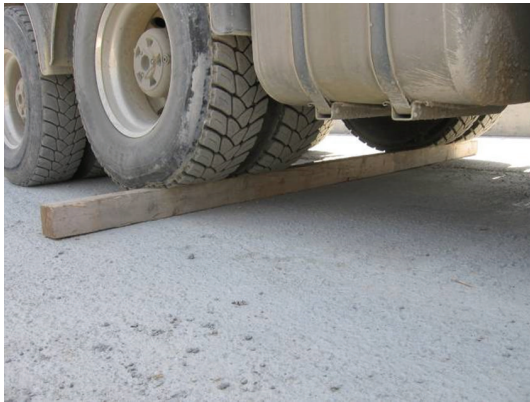
FIGURE 14: Dynamic stimulus of the bridge deck.
