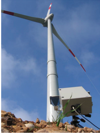
FIGURE 7: Radar measurement of a wind tower.
