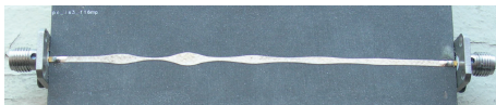
FIGURE 11: Photograph of a microstrip pulse shaper for UWB radar and communication systems.
