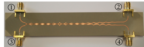
FIGURE 3: Photograph of the fabricated EBG microstrip directional coupler with high directivity and coupling. The ground plane is unaltered.
