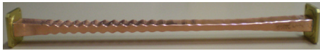
FIGURE 18: Photograph of the fabricated filter prototype in rectangular waveguide technology. Standard WR-90 ports are used.
