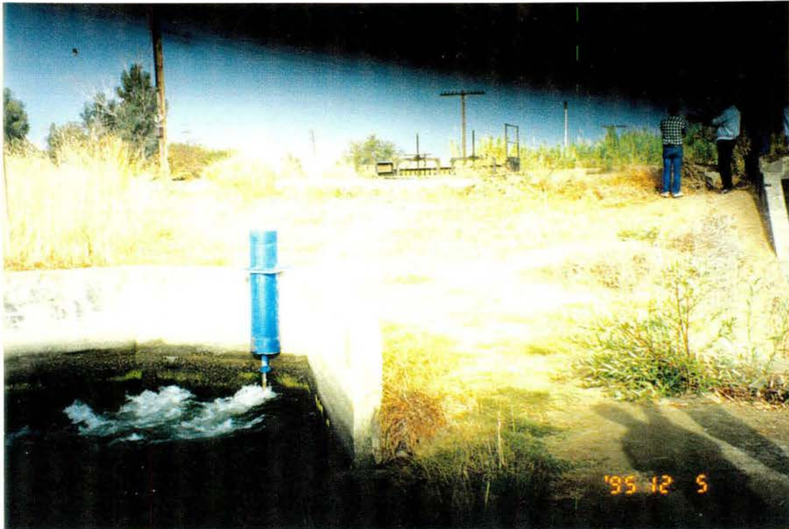
Photograph 5. - Lateral 26.2 - Micrometer propeller flowmeter. Flow measured in one of two outlets to FWS refuge and lateral.
