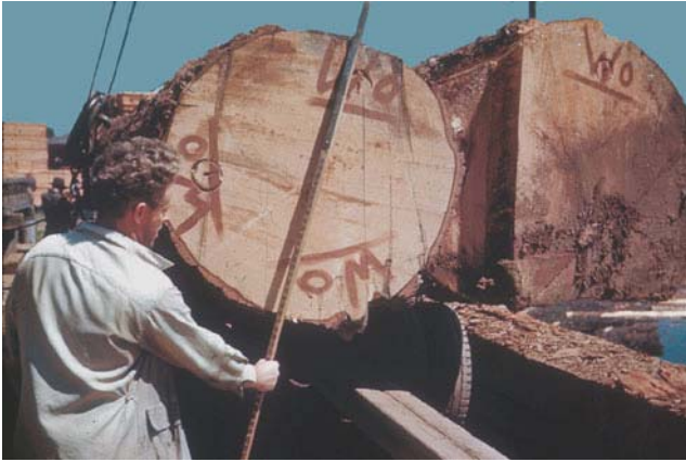
Figure 1—A mill stamp (near the scaler’s forehead) was hammered into the ends of logs to identify log ownership at water sorting grounds.
