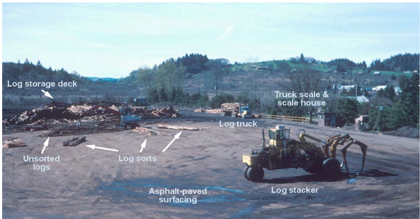
Figure 15—Overview of a paved log sort yard. Note sorting bay, log truck approaching truck scale, and log stacker ready to unload the truck in a single pass, lifting the entire load off.
