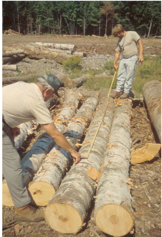
Figure 10—Workers determining whether birch sawlog could be upgraded to a veneer log if it were bucked.
