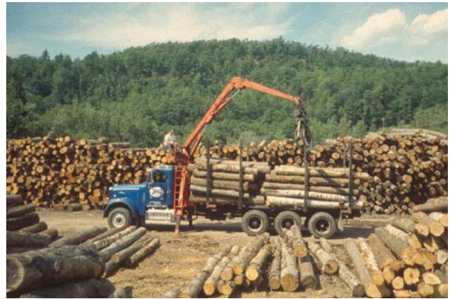
Figure 16—Log-truck-mounted loader typical of hardwood logging trucks.
