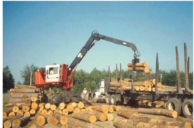
Figure 8—Rubber-tire-mounted hydraulic loader unloading and spreading logs for grading and scaling.
