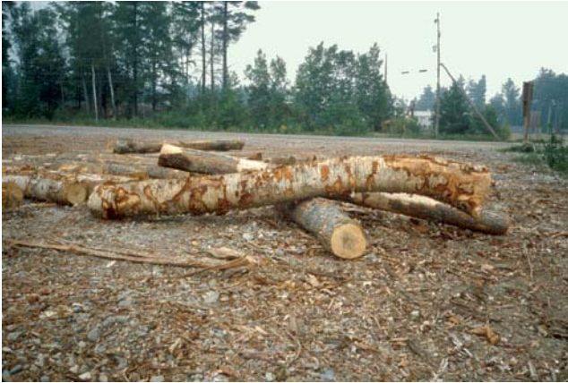
Figure 11—Pistol butt—a poor log-making practice. Proper log making in the woods goes a long way to recovering highest value for the log sort yard operator. This log may be no value because it was mismanufactured.
