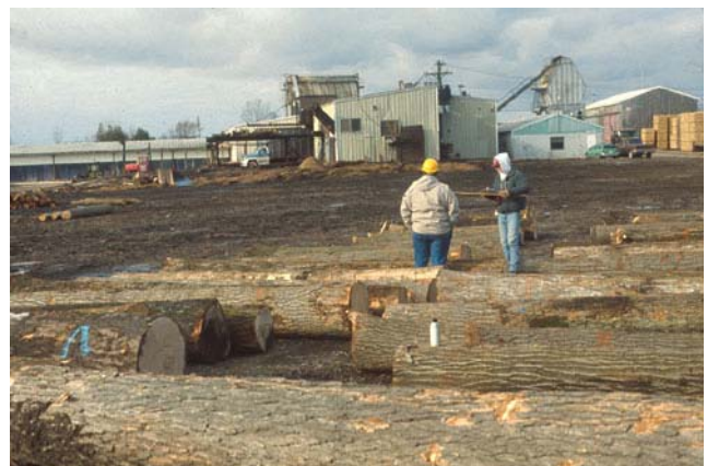
Figure 4—Hardwood sawmill's log yard with logs outspread. Veneer buyer is marking and scaling logs.
