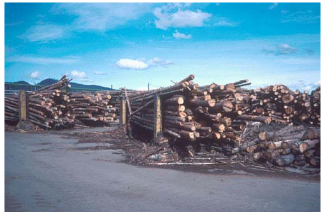
Figure 22—Log sorting bunks to accumulate sort logs for transport by larger machines like a large-capacity front-end loader.
