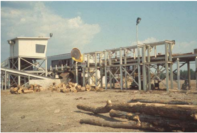
Figure 19—Laser scanning and computer-controlled bucking at a high production log sort yard. The merchandiser bucks logs into various sawlog products, railroad tie logs, and pulpwood.
