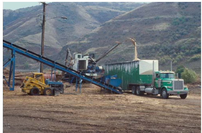
Figure 5— Satellite chipmill yard chips low-grade pulpwood into higher value chips for shipment to pulpmill by chip van.
