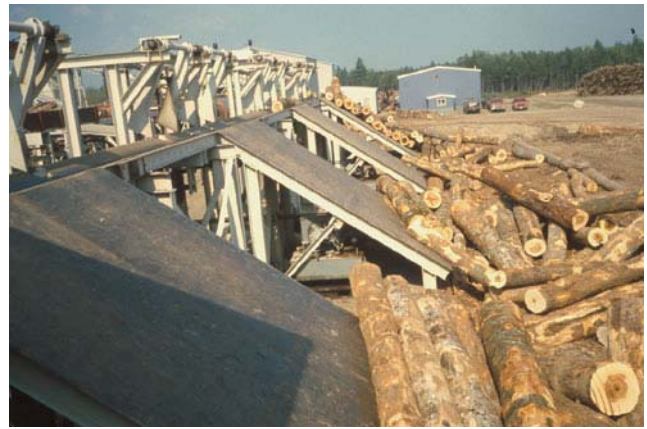
Figure 21—The four sorted log bays as viewed from the log merchandiser grading station.
