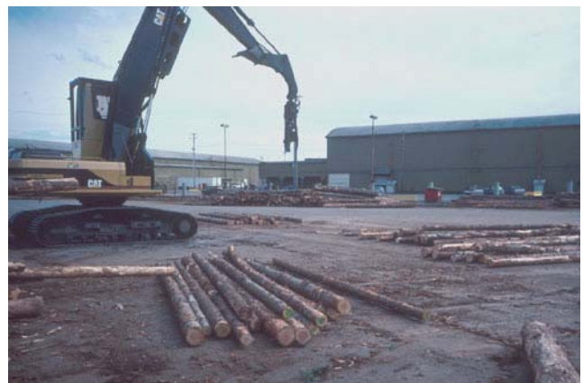
Figure 17—Stationary log loader with sorts laid out on three sides of a square for efficient sorting. Front-end loaders feed logs to the loader for sorting on the fourth side of the square.
