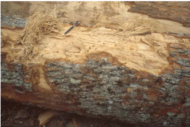
Figure 12—Log fork damage from a front-end loader caused by carelessness or excessive log handling.
