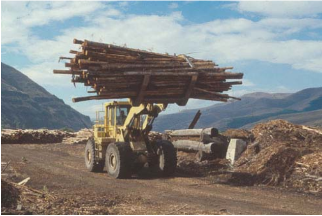
Figure 9—Front-end loader using full machine capacity to transport logs in the yard. Front-end loaders are good multipurpose machines for unloading and reloading, transporting, spreading, and sorting logs.
