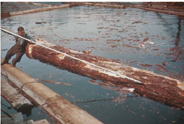
Figure 2—Water sorting logs was done manually using a pike pole.
