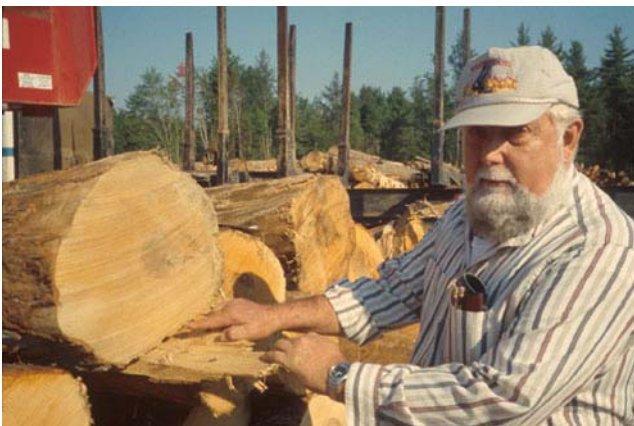
Figure 13—Timber processor damage on a sawlog. Harvesting damage such as splits results in poorer lumber recovery and loss of log value.
