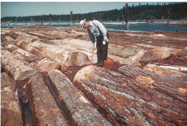
Figure 3—Scaling logs in a log raft ready for shipment down river to the mill.
