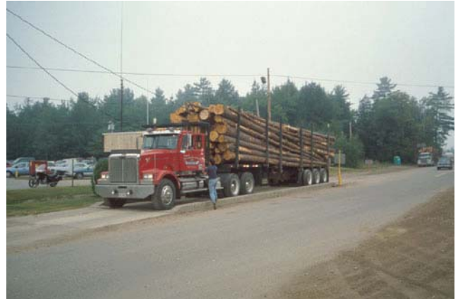
Figure 14—Loaded truck at a large sort yard gets weighed in. After unloading, the truck is reweighed empty and the net log weight is calculated.
